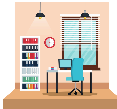
Figure 6B : Potential risk of glare due to improper position of the light source and windows
